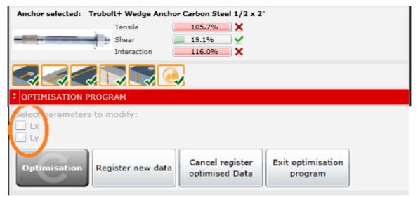
Once the parameters to be modified have been entered, click on Optimization so that RED HEAD TRUSPEC can optimize these values to find a solution for the selected anchor.
