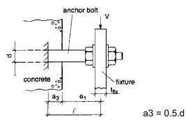
3. Mounting with spacing and nut against the concrete. In this configuration, select the following icon:
