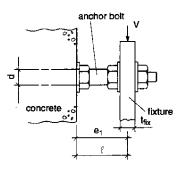
4. Mounting with spacing on an intermediate layer of resurfacing. In this configuration, select the following icon:
