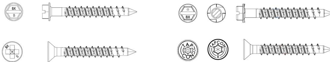
FIGURE 2—TAPCON ANCHORS WITH ADVANCED THREADFORM TECHNOLOGY ANCHORS
