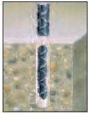
Doweling into Concrete with Rebar
