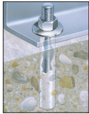
Fastening to Concrete with Threaded Rod
